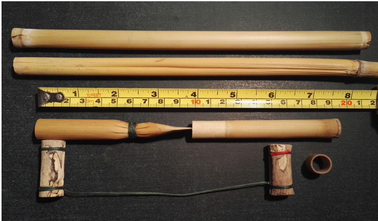
Figure 1: Pair of reeds for a “Megara” aulos in mid-manufacture, 30 August 2019, made by Barnaby Brown using Phragmites australis harvested on Camí de Can Alegria, Palma de Mallorca, 4 July 2019. Top to bottom: Internode with leaf-sheath attached; internode with leaf-sheath removed and wrinkling (useless for reed making); root-end reed with unscraped stem, waist binding, bulge, and scraped blades (removing epidermis and cortex); tube partially scraped to make the partner reed, retaining the flower-end node at the reed exit; driftwood reed caps to ‘educate’ and protect the blades; offcut showing wall thickness of 1.1–1.2 mm. External tube diameter 13.0–13.5 mm; waist internal diameter 4.5 mm; length of scrape 23 mm; tip to top of waist binding 34 mm; total reed length 97 mm. For further details and images, see Brown 2019. © B. Brown.
