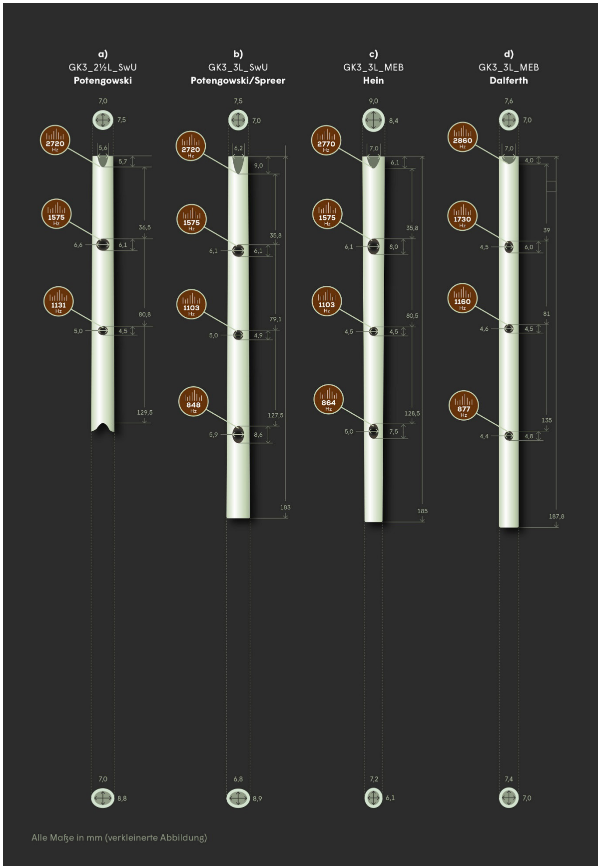
Figure 24: Four reconstructions – measurements and frequency numbers. Design by Matthias Kraus.
