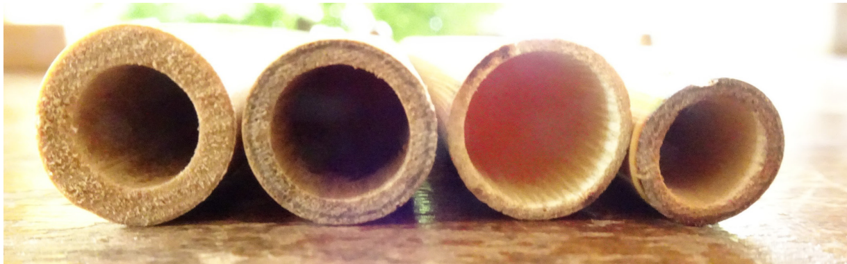
Figure 4: Cross sections showing variability in the thickness of walls, peripheral cortex fibres, and inner xylem tissue of Arundo donax and Phragmites australis growing in different environmental conditions. Left to right: Sardinian Arundo selected for a pipe body; Phragmites harvested at Lago di Nemi, Rome, at Calore Irpino, Benevento, and at Lago Vadimone, Orte. © M. Sciascia.
