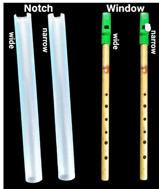
Figure 12: Coverage of the blowhole by construction, left: two tubes with a narrow and a wider notch; right: pennywhistle with a narrow and a wider window. © G. Dalferth 2023.
